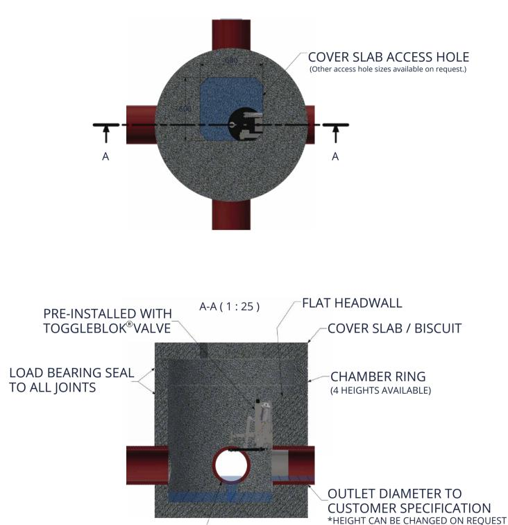
INLET DIAMETER, POSITION AND –/ HEIGHT TO CUSTOMER SPECIFICATION \*3 INLETS MAXIMUM\*
